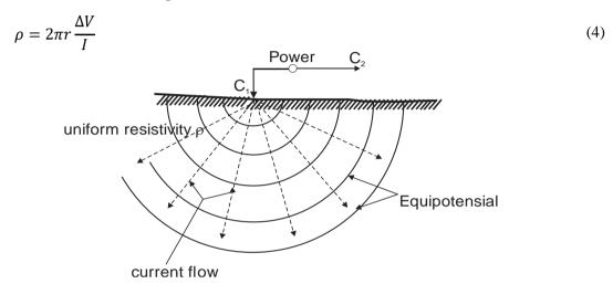
Figure 3 Current source point on the surface isotropic homogeneous (modified from Telford et al., 1990).
