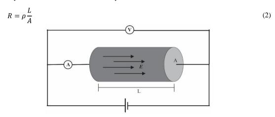
Figure 2 Current flow on cylinder conductor (modified from Margaworo, 2009)
