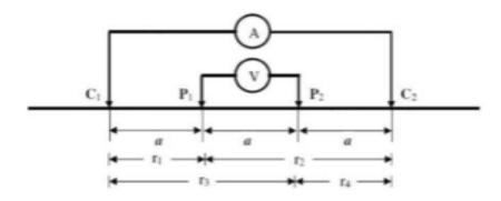
Figure 5 Schematic of electrodes in Wenner configuration resistivity (Reynold, 1997).
