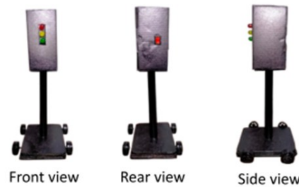
Figure 3. Front, rear (control panel), and side views of the portable traffic light prototype
