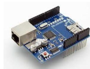
Gambar 4. Modul Ethernet Shield W5100
