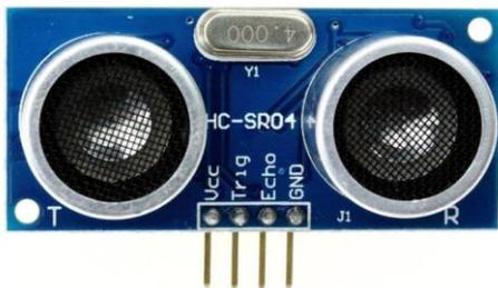
Gambar 2. Sensor Ultrasonik
