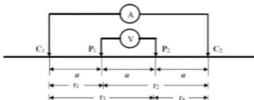
Figure 5 Schematic of electrodes in Wenner configuration resistivity (Reynold, 1997).
