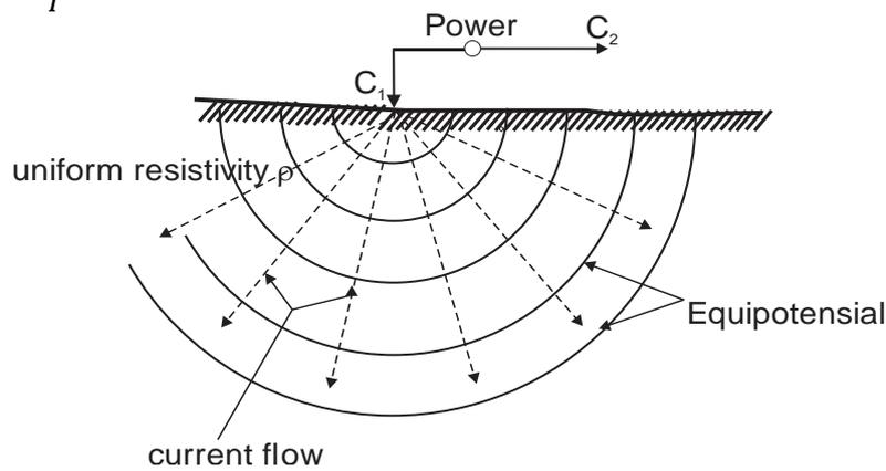
Figure 3 Current source point on the surface isotropic homogeneous (modified from Telford et al., 1990).
