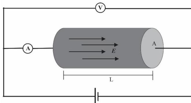
Figure 2 Current flow on cylinder conductor (modified from Margaworo, 2009)
