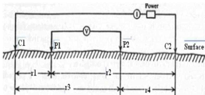
Figure 4 Two current electrodes and two potential electrodes on resistivity measurement (modified from Telford et al., 1990).
