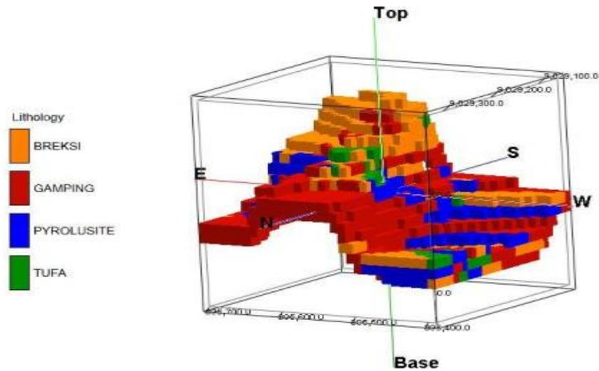
Figure 10 3-D visualizations results of all lanes using software RockWorks 15 in Empol sub-village, Central Sekotong
