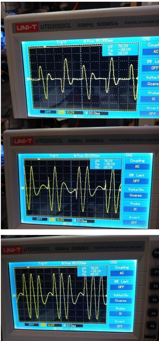
Figure 10. The output waveform of the TRIAC when the PWM duty cycle is 40%, 60%, and 80% as measured with an oscilloscope.
