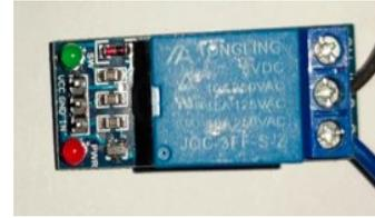
Gambar 4. Relay 1 Channel
