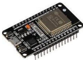
Gambar 4. NodeMCU ESP32
