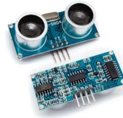
Gambar 2 Sensor Ultrasonik HC-SRF04
