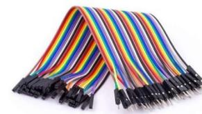
Gambar 9 Kabel jumper
