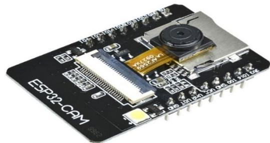
Gambar 1 Esp32-cam
