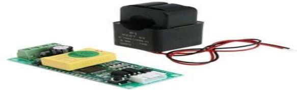
Gambar 3: Modul Sensor PZEM004T
