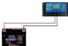
Gambar 10 Solar Charge Controller (SCC) ke Aki
