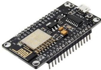
Gambar 1. NodeMCU Esp8266
