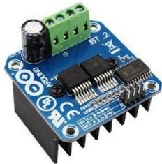
Gambar 7. Driver Motor BTS7960
