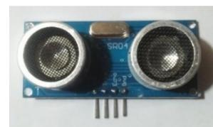
Gambar 3. Sensor Ultrasonik
