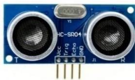
Gambar 3. Sensor Ultrasonik 7.
