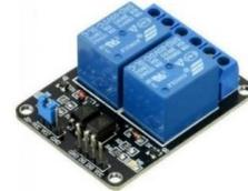
Gambar 4. Modul Relay DC
