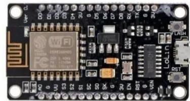
Gambar 1. Board NodeMCU ESP8266
